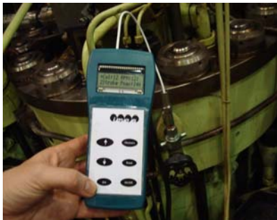
The IMES type EPM-XP electronic engine indicator for diesel engines connected to a notebook for data download. The type HTT sensor and flexible pipe with thompson adaptor are visible on the left.
