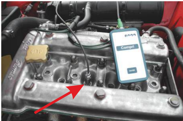
Compri pressure sensor installed on a cylinder of the Alfa GT1300 engine
