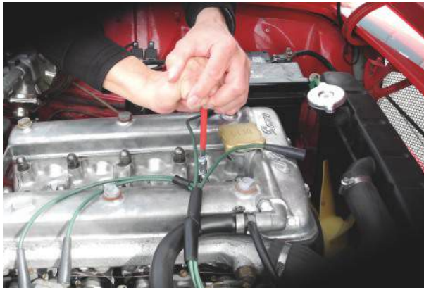
Dismounting of spark plugs on an Alfa GT1300 engine
