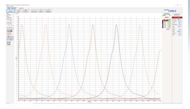
Besides the user has the possibility to save the latest 40 (80) cycles manually under different load or different environmental conditions, e.g. during shop test, sea trial or voyage. He can use the recorded data for later comparison or analysis of engine performance und various conditions. The CCM event record enables to analyse the data before, during and after failure. So, it is possible to determine the cause of failure and to find solutions how to prevent in the future.
