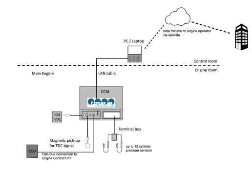
The CCM system can be directly installed at the engine. A sophisticated plug- and play concept enables an easy fitting of cylinder pressure sensors and pulse inputs to the CCM housing.
