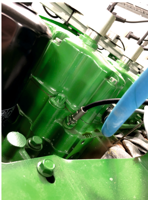
CPS-03 installed on a hydrogen engine
