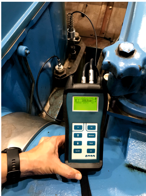
EPM-XP plus-vibro installed on a MAN 12V 48/60 engine at the Endesa powerplant in Melilla
