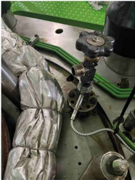
TCS-01CA-PMI sensor installed on a MAN ME two-stroke diesel engine
