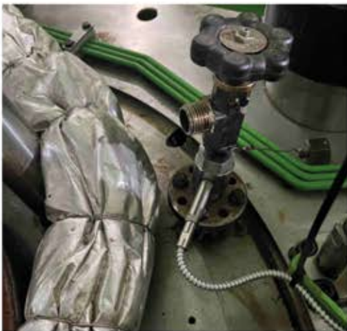
TCS-01CA-PMI sensor installed on a MAN ME two-stroke diesel engine
