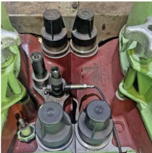
CCM and sensors type HTT-10 installed on a 4-stroke diesel engine for continuous operation.
