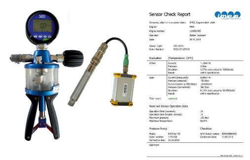
All data will be displayed in a sensor evaluation report and the measured data of sensor offset and -span will be compared with sensor specification.
