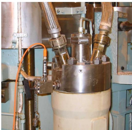
High pressure sensor designed for pressure measurements in hydraulic systems;
