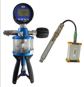
In conjunction with the hydraulic pressure pump including manometer the check-box is suitable for sensor offset and -span evaluation at ambient temperature.
